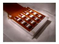
Copper holder for 4 Delrin (POM) crystal layers (16 crystals per layer)
